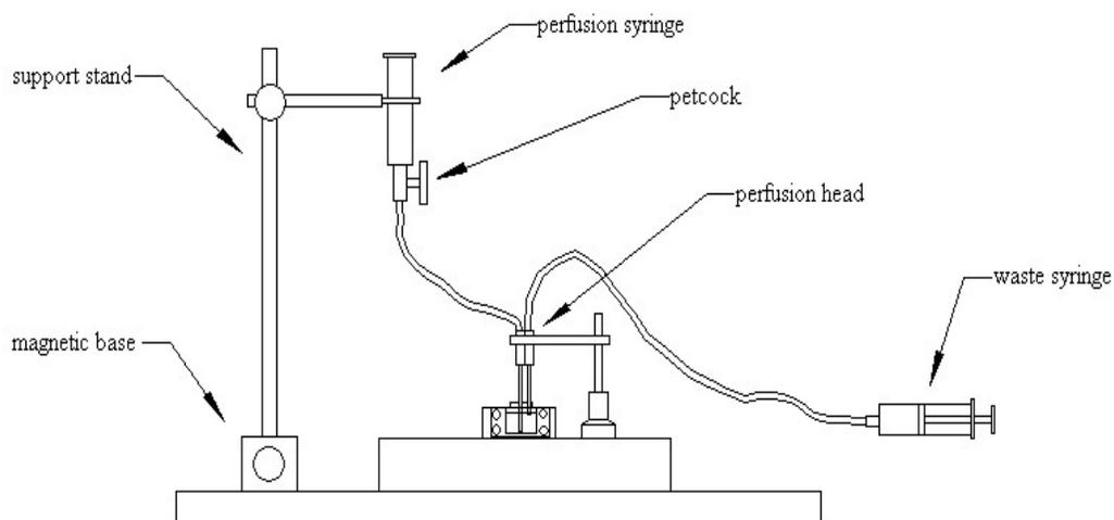
**Note:** In the following assembly instructions, it is important for the input side (reservoir and line) of the perfusion system to remain inside the Faraday cage since the conducting solutions within these components can act as radio frequency (RF) leaks. The requirement for a vacuum aspiration path to be contained entirely within the cage is less stringent since the aspirator generally keeps the line clear of conducting fluids when not in use.
