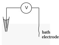
If [Cl<sup>-</sup>] were the same at each of the silver wires, we would expect no potential difference by the symmetry of the system. More typically, the microelectrode is filled with 3 *M* KCl while the bath electrode is immersed in physiological saline, say 150 m*M* NaCl. Setting the ratio of the rates (eqn. 3) to unity for each electrode we have
