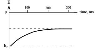
Thus if you wanted to control the membrane potential by applying the commanded potential V to the microelectrode, you would not be very successful: *E* would only follow half the magnitude of the changes you impose, and will follow the changes very slowly, with a time constant of 100 milliseconds. To get around these severe limitations one uses the voltage-clamp techniques that we will consider in the next two lectures.
