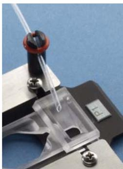
specimens or optical fields to fluctuate during imaging and recording. This approach allows for very smooth solution delivery. I-V perfusion lines can be used to deliver drops at a fixed rate to the chamber without introducing noise into the specimen field. In addition, multiplexed solution delivery is possible without the potential of solution switching artifacts.
