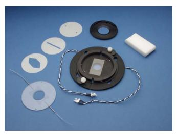
chamber allowing it to be inverted in the mounting platform facilitating its use with both inverted and upright microscopes. An optional heater model is available.
