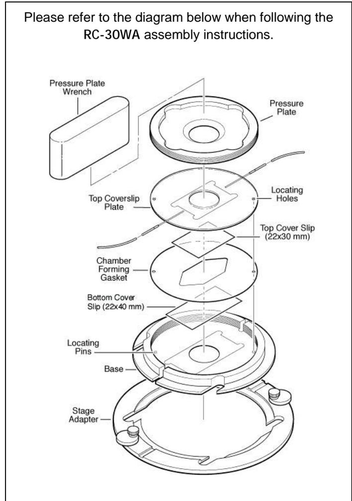
3. Carefully remove the polyethylene cover from the exposed bottom of the gasket taking care to not disturb the existing seal.
