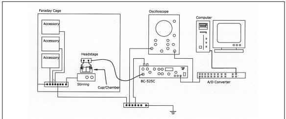
**Figure 2a. Central node grounding scheme.** Note the grounding block within the Faraday cage is connected to the external star ground point and the headstage is not externally grounded.
