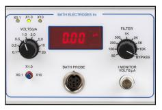
selects the gain multiplier (x0.1, x1.0 and x10). LED's indicate the gain multiplier selection. The combination of these controls allows gain to be set from 0.01 to 200.
