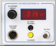
to determine the internal resistance of the voltage probe. When the pushbutton is depressed, a constant 10 nA current is passed through the voltage electrode producing a voltage drop of 10 mV/M $\Omega$  of probe resistance. The measured potential is displayed by the meter or reported at the V<sub>m</sub> x10 output BNC (at 100 mV/M $\Omega$ ).
