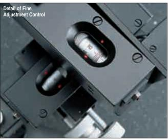
These micromanipulators provide 'hands off' control for fine adjustments. Each axis has a controller motor with a flexible coupling to the micrometer spindle which ensures that the probe can be moved with zero vibration.
