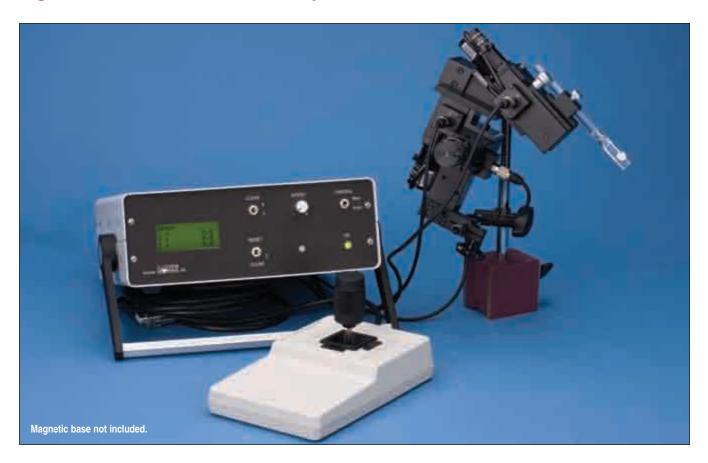
The SM-3 is a high-resolution, three axes motorized micromanipulator featuring a compact design, 25 nm resolution, and a low noise controller. Linear amplifiers, used to drive the stepper motors, eliminate stray electromagnetic radiation, a key feature for patch clamp and noise sensitive electrophysiology applications.
