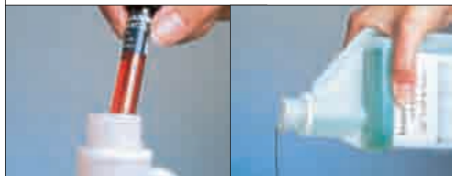
Step 3. Insert electrode for calibration.
