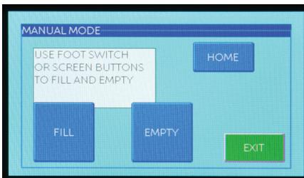
If the [FILL] or [EMPTY] icon has been pressed and you desire to stop the action, simply press the same icon position (now labeled [STOP]) a second time.
