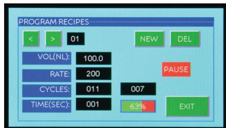
Below the **[RUN]** icon is a box displaying the number of injection cycles remaining in the entire program recipe. It will count down toward (0) as the multiple injection cycle progresses. Below this "counter" box is a display of the percentage of the program recipe remaining. It will count down toward (0%) as the multiple injection cycle progresses.
