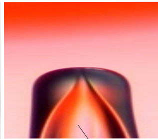
Pipette cavity expanded by air pressure
