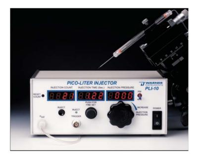
The **PLI-10** Pico-liter Injector is designed to provide controlled delivery of picoliter to nanoliter volumes of solution through a glass micropipette. The **PLI-10** is ideal for applications such as neuronal tract-tracing, delivery of pharmacological agents in vitro, and *Xenopus* oocyte injection.
