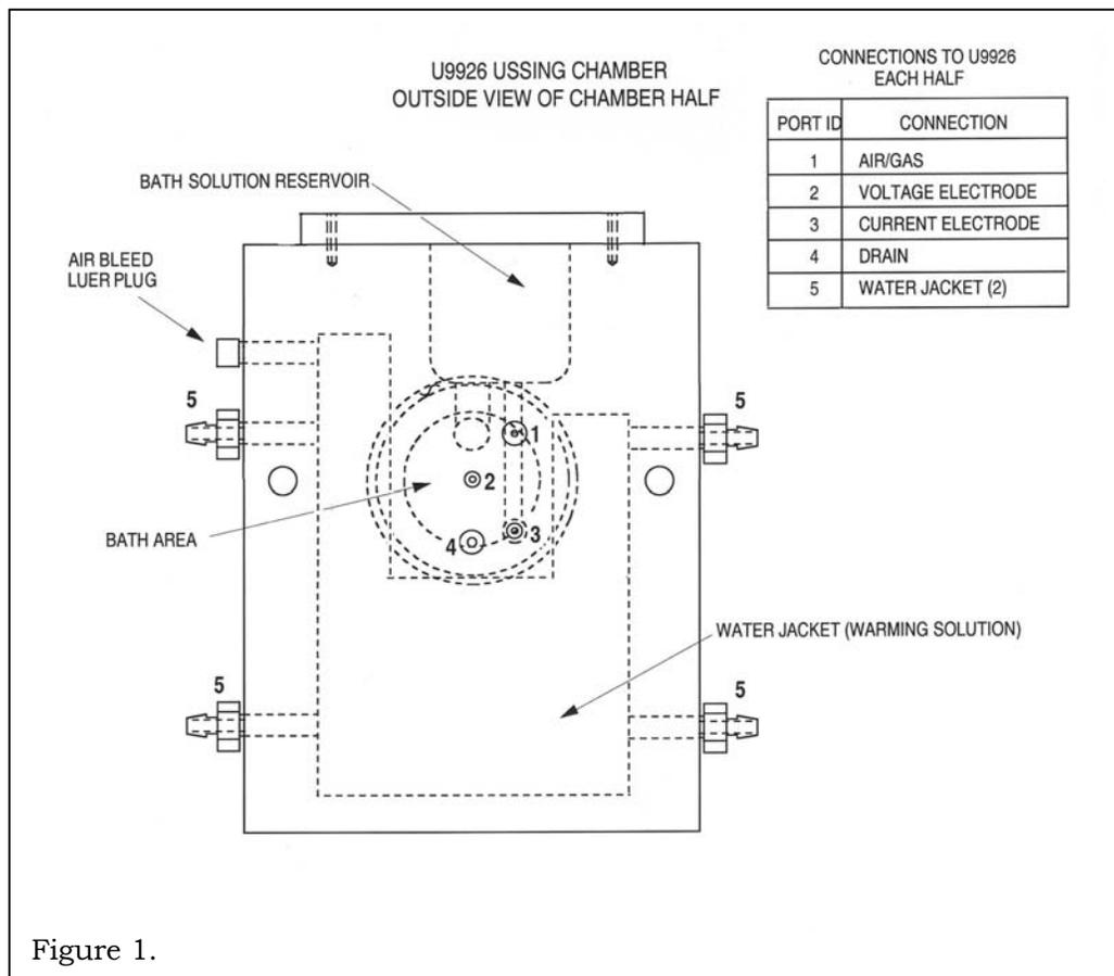
Ports 1 and 4 are Luer taper holes which accept standard male Luer fittings that have been shortened in length by 3 mm. Any standard plastic male Luer fitting can be made acceptable by removing 3 mm from the length.
