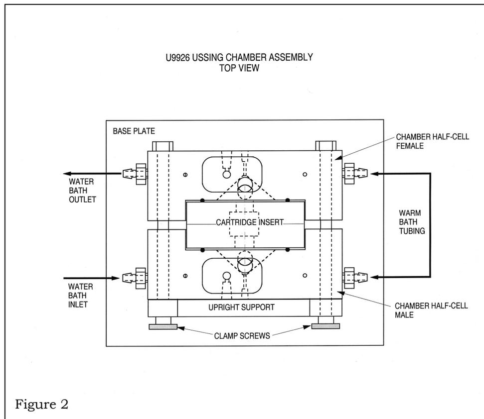
2. Place the cartridge inserts into the loosely assembled chamber halves (note that the large hole is on the bottom and will align with the center of the chamber when inserted). After inserting the cartridges, securely tighten the screw clamps but do not over-tighten.
