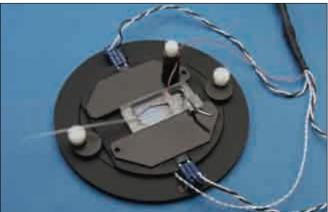
RC-22 shown in a PM-1 heated platform
