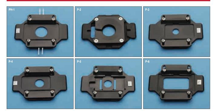
The Warner Series 20 platforms function as a base for Series 20 chambers and provide clamping to make a seal between the chamber and coverslip. Platforms are machined from aluminum and finished with a black anodize. This provides excellent heat conductivity and minimizes stray light reflectance. Platform designs are optimized to provide maximum heat transfer to the coverslip and still afford excellent access for objectives.
