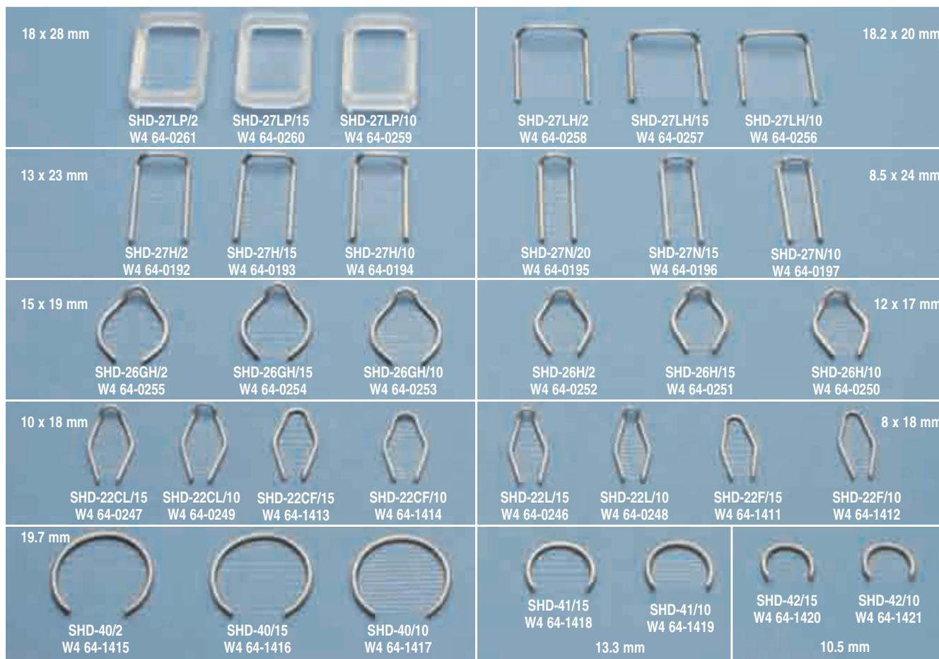
Slice anchors are available for most open bath chambers in the 20 and 40 Series family except for field stimulation chambers. Anchors are constructed for an easy push-in fit into the chamber's bath area. This allows the user to control the anchor pressure applied to slice. Most anchors are made from type 316 stainless steel and Lycra® and finished with a plastic coating. Plastic anchors are available for the RC-27L Chamber.
