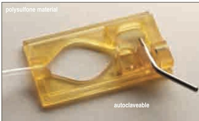
All Series 20 chambers equipped with a stainless steel suction tube now include a suction tube clamp. This insures the adjustable tube will not move once the solution height is set.
