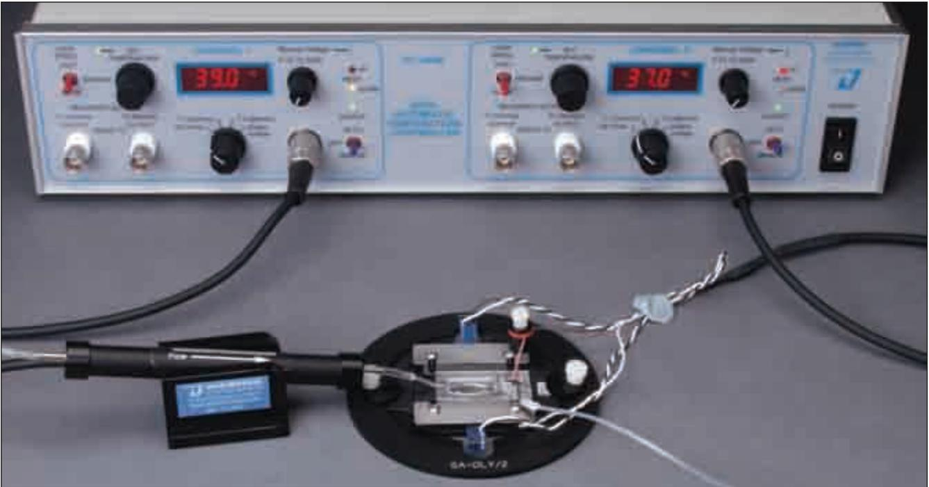
Shown above is a typical complete system, which includes an RC-22 chamber, heated platform, dual channel temperature controller, in-line solution heater, connecting cable and a stage adapter.
