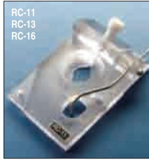
These chambers are open bath chambers suitable for physiological experiments performed with inverted or dissecting microscopes, including patch and oocyte recording, isolated perfused tubule, and cell impalement studies. RC chambers have also been used with fluorescence microscopy.
