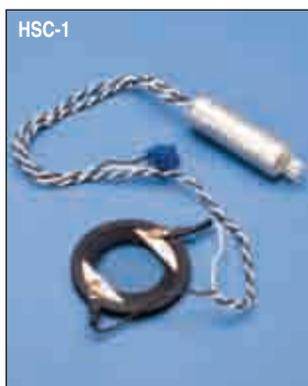
Developed for use in our DH-35i and DH-40i Micro-incubation chambers, this heated coverslip assembly replaces the 40 mm coverslip normally supplied with these chambers. Once installed, the HCS-1 eliminates condensation which occurs when these chambers are used in the closed mode.
