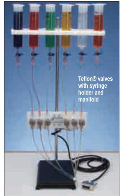
Teflon® valves with syringe holder and manifold
