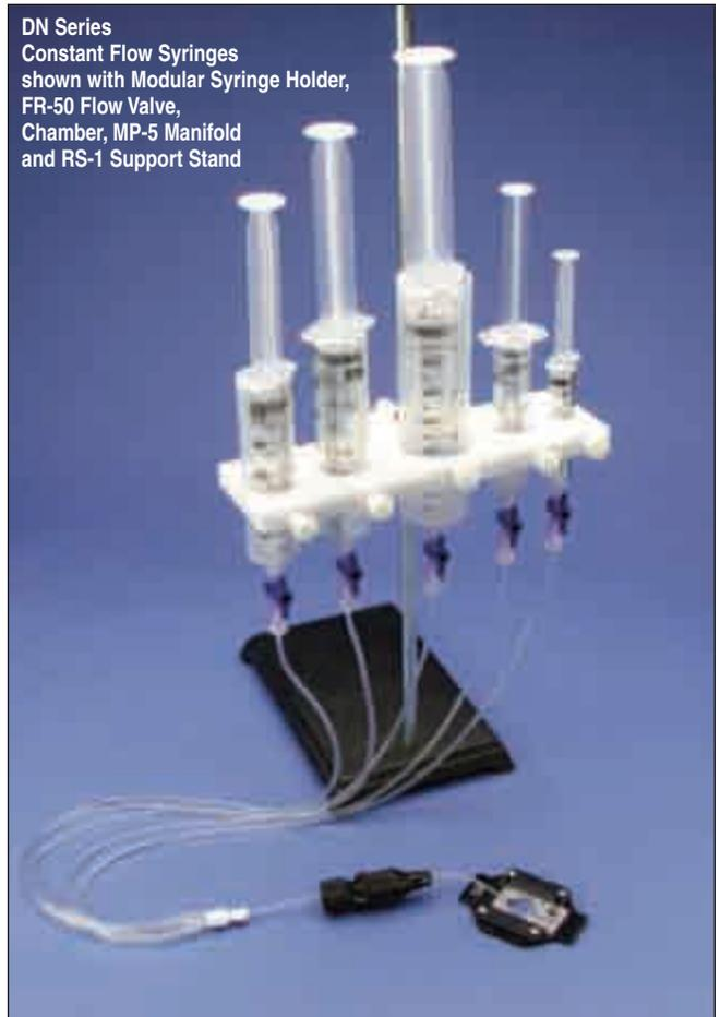
When using a gravity-feed perfusion system, a common difficulty facing researchers is maintaining a constant flow as the reservoir empties. In general, since head pressure is a linear function of column height, the change in height of a 60 cc syringe as the solution reservoir drains can result in as much as a 20% decrease in flow rate.
