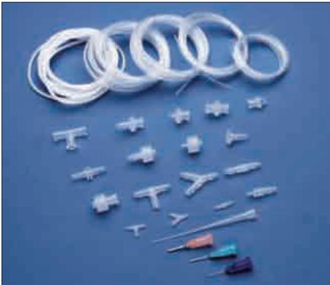
Warner Instruments offers a complete tubing and connector kit. This kit is ideal for use with Warner's Imaging and Recording Chambers. The kit is comprised of barbed and Luer fittings, blunt end needles, and an assortment of PE and C-Flex tubing. All barbed and Luer fittings are made from polypropylene and include tube to tube, reducing, Y-, T-, Luer-to-Luer, and Luer-to-barb adapters.
