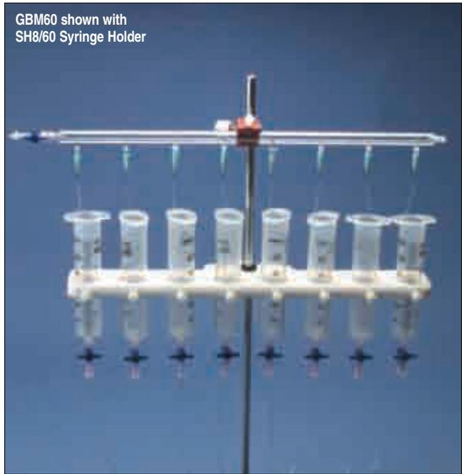
These gas bubbler manifolds for 10 and 60 cc syringes are useful for delivering water soluble gases to syringe reservoirs mounted in Warner syringe holders. Luer fittings on all the inlet and outlet ports make these manifolds very easy to assemble. Constructed from clear polycarbonate for durability and easy cleaning.
