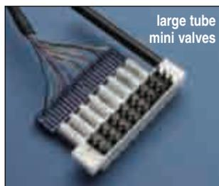
While pinch valves are standard equipment, additional valve options include Teflon and Lee miniature types. The VC-8M is designed for slow flow perfusion systems where smaller diameter tubing is used. The VC-8MLT uses larger ports on a mini-valve platform to accommodate the PE-160 tubing used on most Warner chambers, this version will permit flow rates of up to 10 ml/min.
