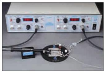
TC-344B – Dual Channel temperature controller shown with in-line solution heater and heated platform with connecting cable.
