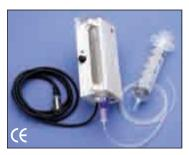
The ability to independently control each heater block allows the researcher to control the initial temperature of each solution without influencing other nearby solutions. This system is available to fit 60 cc syringes. The heater housing is made of anodized aluminum which is both corrosion resistant and serves as
