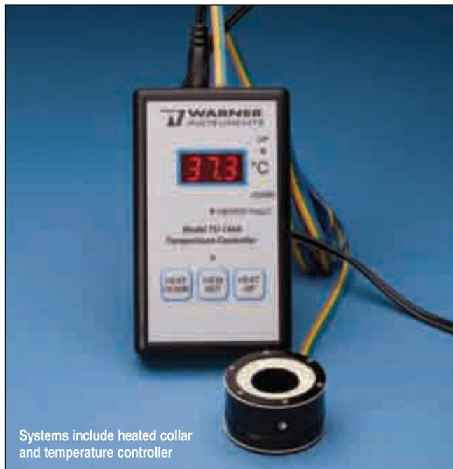
Systems include heated collar and temperature controller
