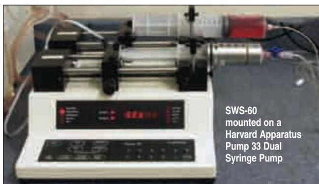
SWS-60 mounted on a Harvard Apparatus Pump 33 Dual Syringe Pump
