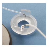
component should be near the top of the clamped 35 mm dish (i.e. roughly 12:00).
