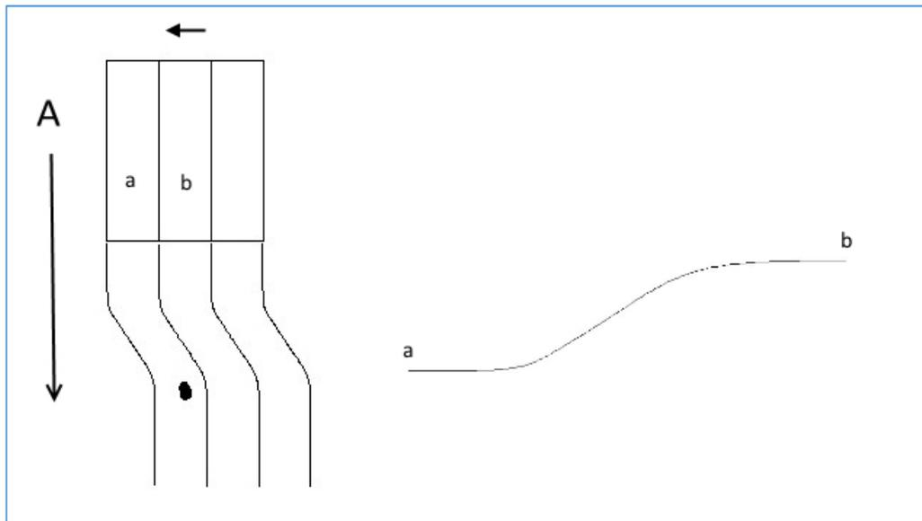
In this example, we have deliberately chosen to step the perfusion tubes sideways at the same speed that the solution flows in the bath. In other words, both the sideways step velocity and overall bath velocity are at speed A. As you can see from the drawing, the a-b boundary reflects this arrangement in that the boundary angle is now 45°. In this case, it will take longer than in the previous example for the boundary to fully cross the cell. This is illustrated in the graph to the right.
