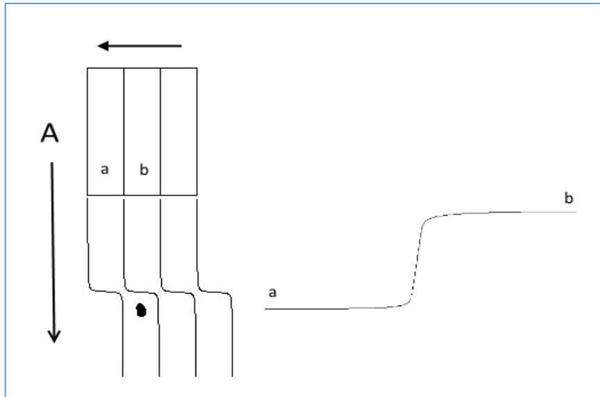
In this example, the sideways step speed is approximately ten times faster than the bath flow speed. As can be seen, the a-b boundary is now almost a horizontal line. (Note that a horizontal line represents the a-b boundary configuration that can sweep across the cell the fastest.) This is illustrated by the graph to the right in this figure.
