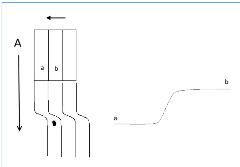
All solutions (including the bath, solution a, and solution b) are flowing at the bath speed A. You can see from the drawing that while the stepper has shifted to target the cell with solution b, this change is still en route and has not yet arrived at the cell. Since all solutions are flowing at the same speed, the boundary between solutions a and b (the a-b boundary) is also moving at the bath flow velocity A.
