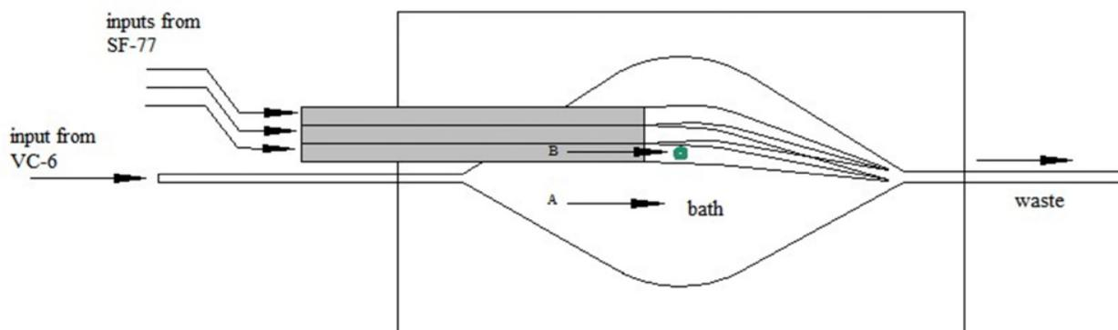
Note that the flow rate in the bath and in the tubes has been adjusted so that the *flow velocity* (or speed) of both is the same (e.g., A and B arrows are the same length). Since the relative speeds are the same, the only mixing is lateral diffusion and the cell (green dot) sees only a single, pure solution.
