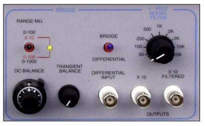
When balanced, the <u>ten turn dial</u> of the DC BALANCE control allows a reading of the electrode resistance. This reading is calibrated to the ELECTRODE RESISTANCE RANGE toggle.
