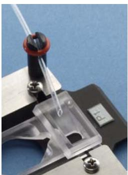
Another feature in common with **JG Series** chambers is the use of a glass coverslip for the floor of the chamber. In most cases, this same coverslip contains the sample. When viewed with inverted microscopes, images are visualized through a single thickness of glass, usually 0.13-0.17 mm.
