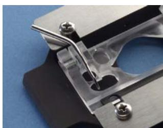
In general, the SS aspirator is installed in a slot in the wall of the suction reservoir allowing adjustment of the fluid level in the main body of the chamber. Adjust (1) the height of the aspirator and (2) the vacuum pressure until the suction rate is equal to the flow rate into the chamber. The basic assembly is shown to the right.
