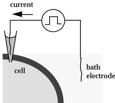
The arrow of current says that net positive charge is moving in that direction. (In the metal wires, actually electrons are moving in the opposite direction). At the wire in the microelectrode the following reaction is taking place
