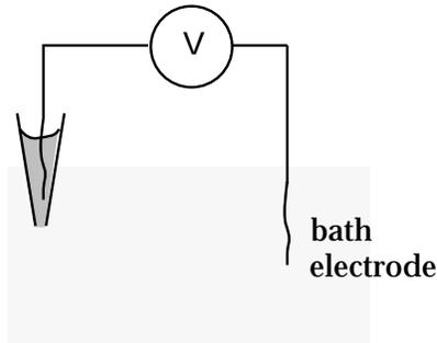
If  $[\text{Cl}^-]$  were the same at each of the silver wires, we would expect no potential difference by the symmetry of the system. More typically, the microelectrode is filled with 3 M KCl while the bath electrode is immersed in physiological saline, say 150 mM NaCl. Setting the ratio of the rates (eqn. 3) to unity for each electrode we have
