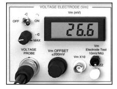
The  $V_m$  ELECTRODE TEST control is used to determine the internal resistance of the voltage probe. When the pushbutton is depressed, a constant 10 nA current is passed through the voltage electrode producing a voltage drop of 10 mV/M $\Omega$  of probe resistance. The measured potential is displayed by the meter or reported at the  $V_m$  x10 output BNC (at 100 mV/M $\Omega$ ).
