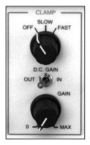
NOTE: All CLAMP controls are disabled by turning the CLAMP MODE SELECTOR switch to the off position. Be sure to switch this control to the off position before handling electrodes!
