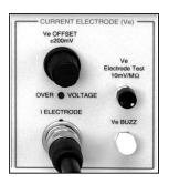
ELECTRODE TEST - A voltage proportional to the resistance of the current electrode [10 mV/M $\Omega$ ] will be displayed on the meter by depressing the ELECTRODE TEST push button when the <u>CLAMP</u> MODE SELECTOR switch is in the <u>off</u> position.
