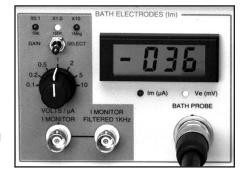
selection. The combination of these controls allows gain to be set from 0.01 to 100.
