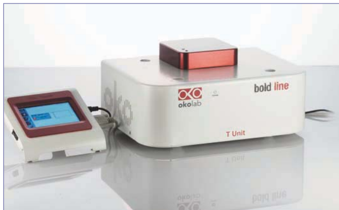
Touch Screen, Temperature Controller and Optional Smart Box
