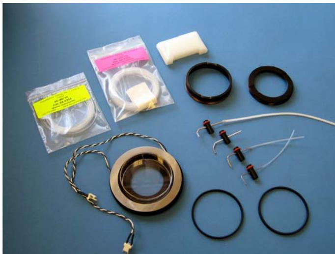
Removable perfusion and suction tubes allow precise perfusion control. Tubes are easily positioned on the magnetic platform. This feature facilitates simple and exact repositioning of both the suction and perfusion tubes following chamber exchange. A newly redesigned suction tube eliminates tidal action and fluid flutter in the bath, resulting in quiet aspiration.
