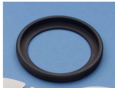
4. Select the appropriate retainer ring for the dish used. The taller ring is used with Corning and Nunc dishes, and the shorter ring is used with Falcon and Willco Wells dishes. Secure the dish into place by screwing the ring into the platform around the dish.
