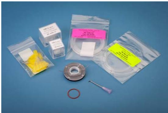
The QR-43C is shipped with an anodized base, the chamber body and a retaining ring to hold the top coverslip in place. Also included are 10 ft of PE-160 tubing, 10 ft of PE-90 tubing and 100 each of 25 and 18 mm round #1 coverslips. The package is rounded out by the inclusion of (12) luer-lock blunt-tip needles, two (2) replacement gaskets and a lift tool for use in removing the
