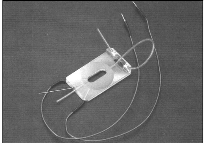
The chamber features an injection port adjacent to the bath solution input port for direct introduction of substances or removal of bubbles. The chamber also features a back-pressure control on the solution output port.
