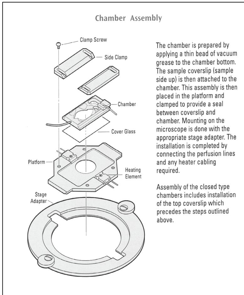
The chamber is prepared by applying a thin bead of vacuum grease to the chamber bottom. The sample coverslip (sample side up) is then attached to the chamber. This assembly is then placed in the platform and clamped to provide a seal between coverslip and chamber. Mounting on the microscope is done with the appropriate stage adapter. The installation is completed by connecting the perfusion lines and any heater cabling required.
