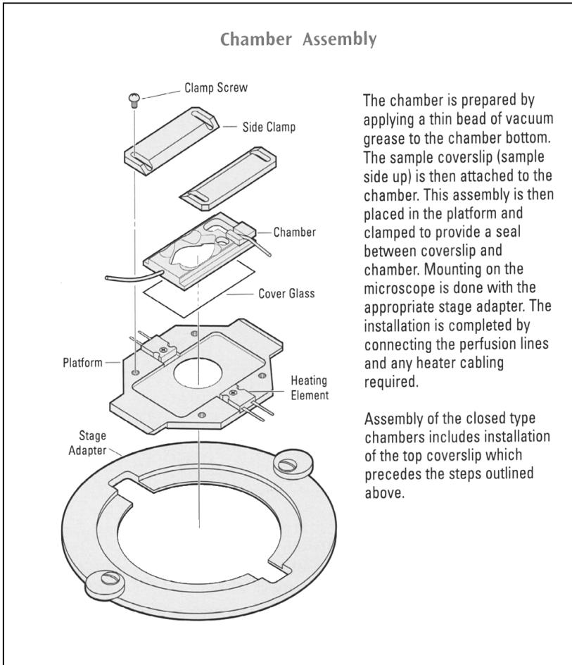
is larger than the platform necessitating the use of a stage adapter. In addition, a stage adapter is highly recommended if the platform is to be heated since it provides insulation between the platform and microscope stage.
