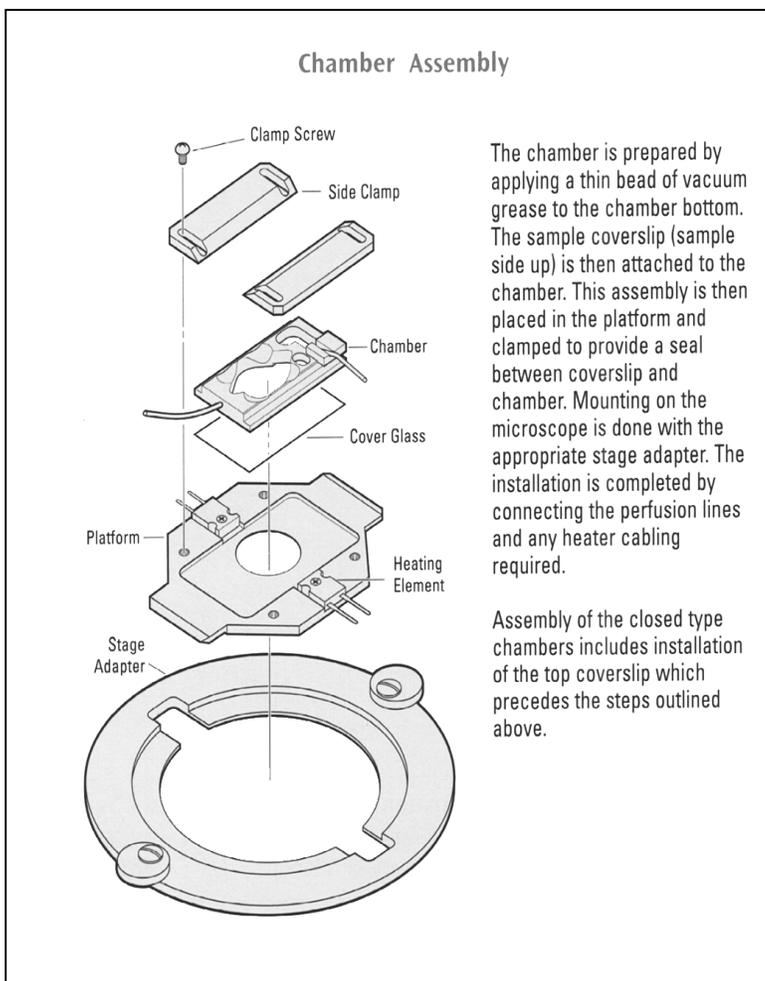
The chamber is prepared by applying a thin bead of vacuum grease to the chamber bottom. The sample coverslip (sample side up) is then attached to the chamber. This assembly is then placed in the platform and clamped to provide a seal between coverslip and chamber. Mounting on the microscope is done with the appropriate stage adapter. The installation is completed by connecting the perfusion lines and any heater cabling required.
