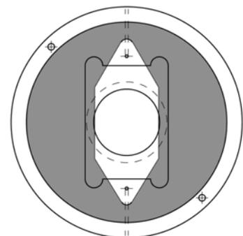
7. Connect a perfusion line to the chamber input and completely fill the bath with solution. Tilting the chamber while filling will help avoid the occurrence of trapped air pockets. Once the chamber is filled, wipe away any excess moisture and place the chamber onto a flat surface. Check for leaks and re-tighten the PRESSURE PLATE if necessary.
