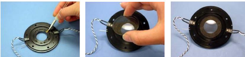
4. Place the coverslip TOP PLATE, with attached gasket, into the PLATFORM BASE while aligning the heater block cutouts (indentations) with the heater blocks in the base. Check for proper fit.
