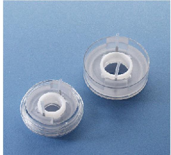
2. Begin by removing the coverslip retainer from the top of the chamber using the pry bar. Remove the installed coverslip. Place aside for later use.
