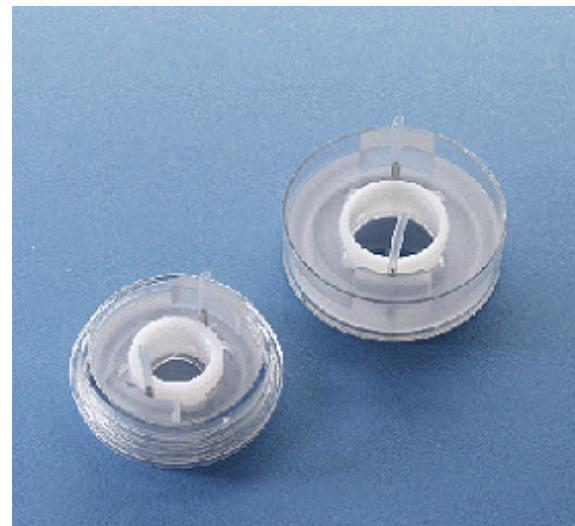
The closed design of the chambers promotes an even and continuous solution exchange with no alteration in focus due to changes in bath height. Studies using gassed solutions can also be performed with no change in partial pressure at the chamber interface. A round coverslip seals the top of the bath resulting in a distance of 1 mm between the top coverslip and culture dish base. The chamber features a hold down ring to secure the top coverslip into place.
