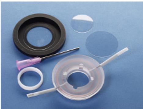
The **RC-43C** is shipped with an anodized base, the chamber body and a retaining ring to hold the top coverslip in place. Also included are 10 ft of **PE-160** tubing, 1 ft of **PE-90** tubing and 100 each of 25 and 18 mm round #1 coverslips. The package is rounded out by the inclusion of two (2) replacement gaskets and two (2) tools for use in removing the retaining ring from the chamber body.
