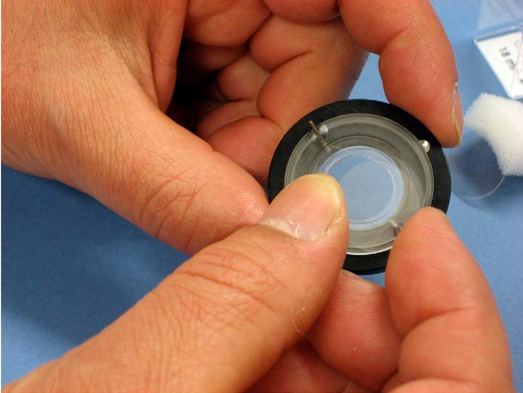
8. Press the white retaining ring into place to secure the top coverslip.
