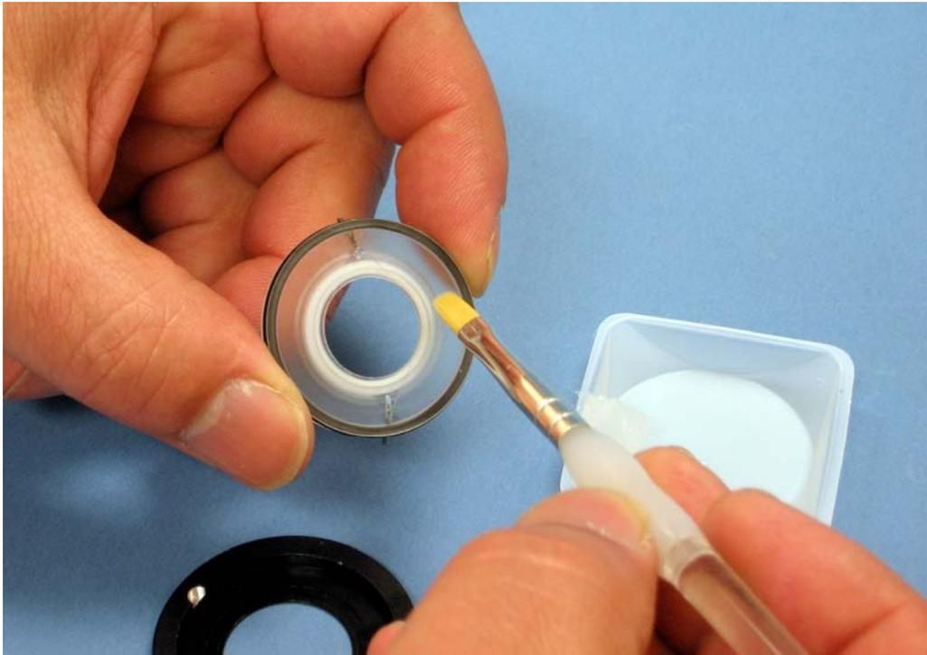
4. Place the bottom coverslip, sample side up (if this coverslip contains the sample), into the recess in the base.
