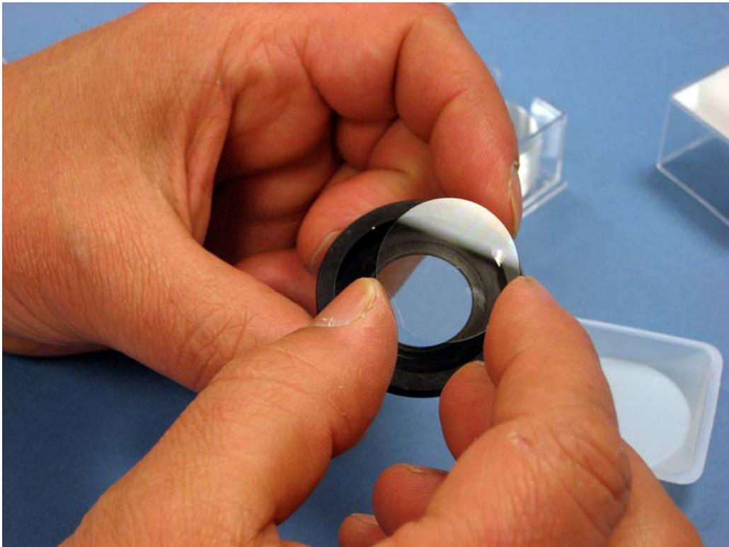
5. Press the greased chamber into the base.
