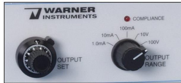
Constant current modes are 0-1 mA, 0-10 mA and 0-100 mA. The desired current is set using the lockable 10-turn OUTPUT SET potentiometer. A red COMPLIANCE LED indicates when the external resistance is too high, preventing the instrument from maintaining the set current value.
