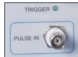
In *bipolar* mode the pulse length of the TTL *high* signal defines the duration of the initial phase of the bipolar pulse. As is expected from a bipolar pulse, the second component of the pulse will have equal duration, but opposite amplitude. If a second TTL *high* signal is applied during the second phase of the bipolar pulse, the first pulse will continue to completion before the instrument accepts the new, incoming signal.
