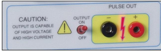
An OUTPUT TOGGLE SWITCH is provided to turn the pulse output *on* or *off* without need to access user settings. In the *off* position, the RED and BLACK OUTPUT JACKS are shorted together.
