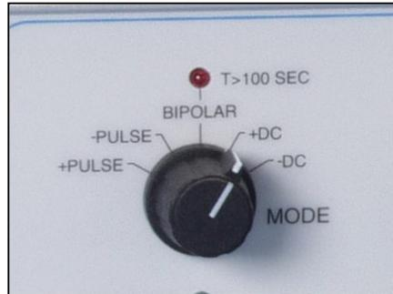
Bipolar pulse widths are user adjustable from 100  $\mu$ s to 100 s and are *per* polarity. A red LED indicates when pulse length exceeds 100 s. The initial polarity of the pulse can be inverted by reversing the connections to the PULSE OUT JACKS.
