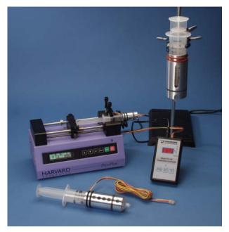
The **SWS Syringe Heater** have two o-rings mounted into grooves in the top of the unit which serve to provide a gripping mechanism for inserted syringes. As a result, a syringe can be partly or completely inserted into the heater body.
