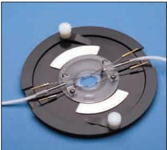
RC-49FS Shown in a Leica Galvo stage adapter
