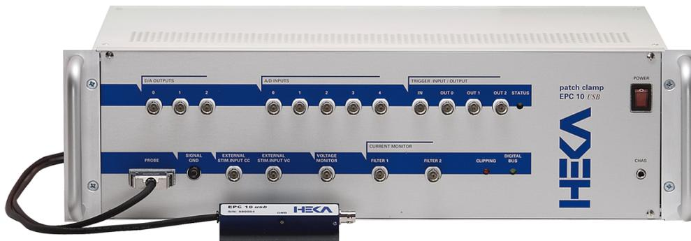
Figure 1.1: EPC 10 USB Patch Clamp amplifier
