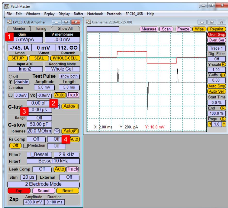
Figure 4.3: Before C-fast compensation
