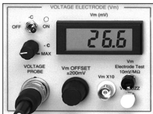
The VOLTAGE PROBE CONNECTOR is a 7-pin DIN connector for attachment of the voltage probe to the instrument.
