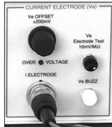
ELECTRODE TEST - A voltage proportional to the resistance of the current electrode [ $10 \text{ mV/M}\Omega$ ] will be displayed on the meter by depressing the ELECTRODE TEST push button when the CLAMP MODE SELECTOR switch is in the *off* position.
