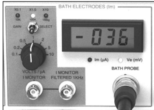
When in clamp mode (CLAMP MODE SELECTOR switch set to *slow* or *fast*), the CURRENT METER displays the current ( $I_m$ ) sensed by the bath electrode. A lit LED indicates current readings in μA.
